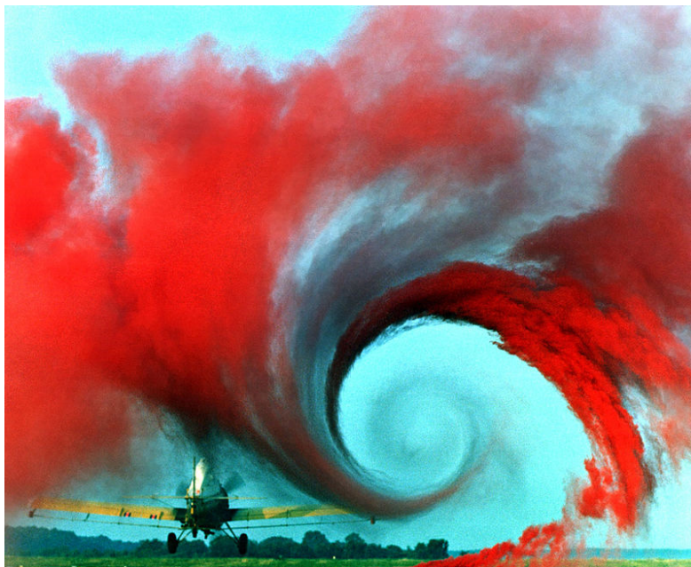
Vortex created by the passage of an aircraft wing
